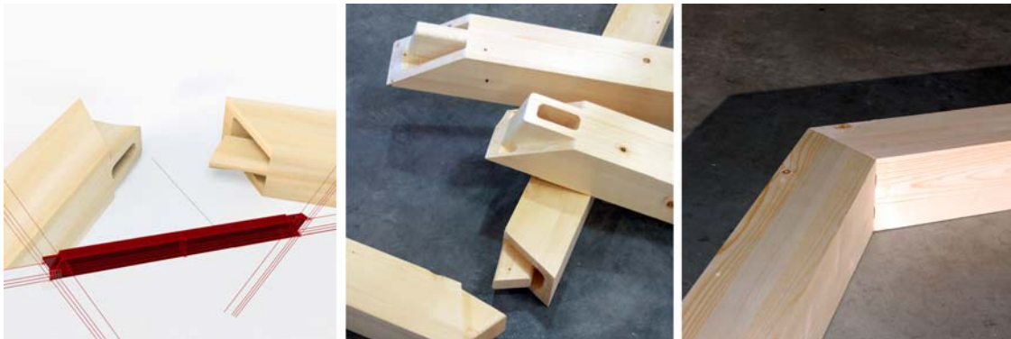
Figure 6 Comparison of digital parametrical model (left), milled joint parts (center) and assembled joint (right).
